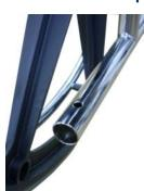
Remove the step tube end cap to expose the two, pre-drilled holes in the frame.
